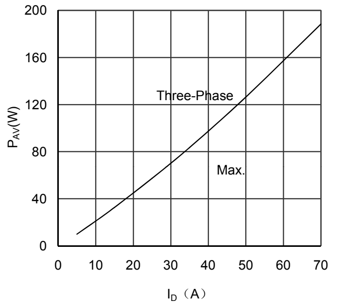
Figure 2. Power dissipation vs Output Current
